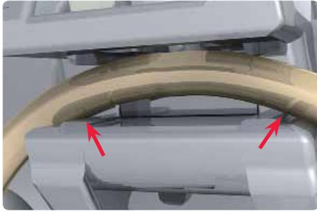
Four contact ribs in the bracket slot ensure controlled force transfer with minimal friction (no binding and notching).
